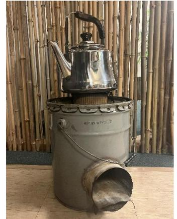
*Note: If metal buckets are unavailable, square cooking oil cans may be used or the entire stove can be fabricated of sheet metal. Dimensions shown are approximate and are dependent upon the actual bucket dimensions.*
